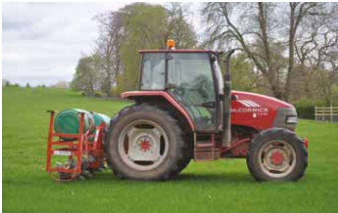
Soil aerator. Image © Eden Rivers Trust
